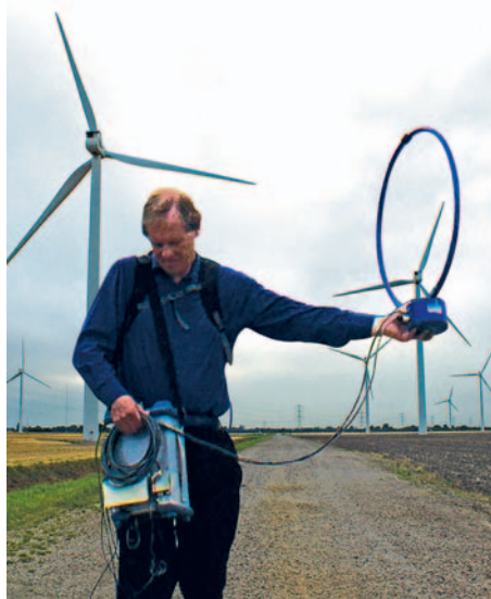
PHOTO 3: Portable EMC measurements at a wind farm.
