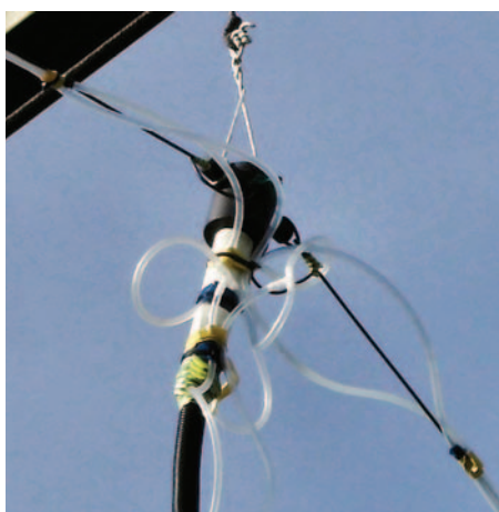
PHOTO 2: Close-up view of the feedpoint. Note how the pairs of tubes are joined by a T-piece to the 'feeder' tube.
