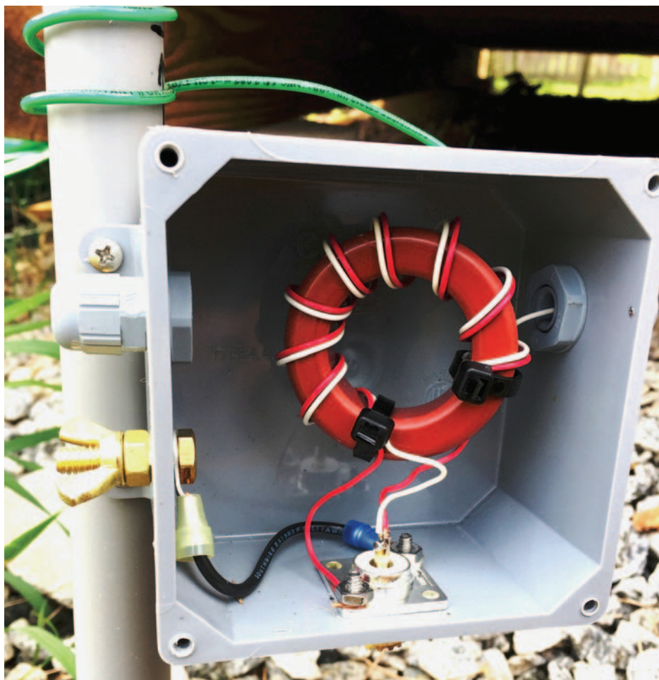
PHOTO 1: WR8RW's 1:4 unun auto-transformer used for matching the helical vertical 20m antenna. The brass wing nut 'common' connection enabled the 1/4\lambda radial to be attached.
