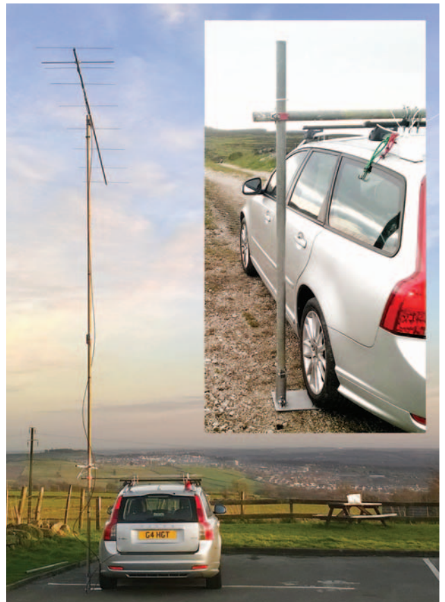
PHOTO 1: My portable aerial mast and 9-ele Powabeam. The inset shows the drive-on plate, stub mast and stabilisation arrangements.
